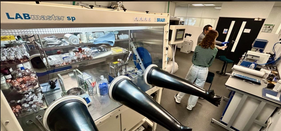
Part of battery cell (coin and pouch) production for in-house testing and QC/QA
