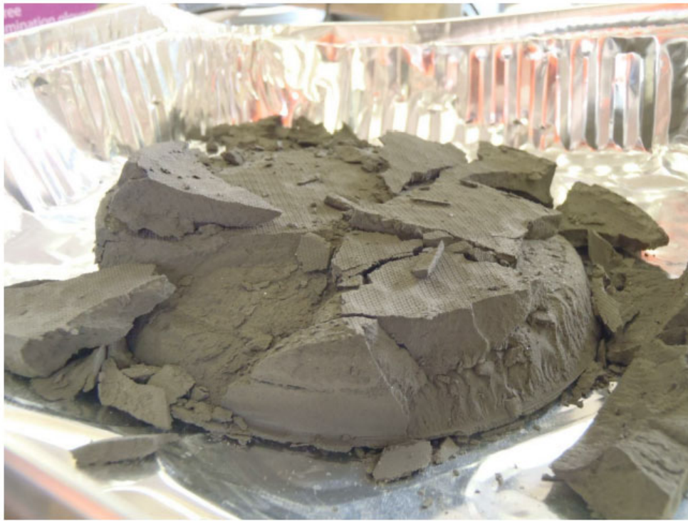
Photograph 6-4 Filter cake with a moisture content of 25.3%
