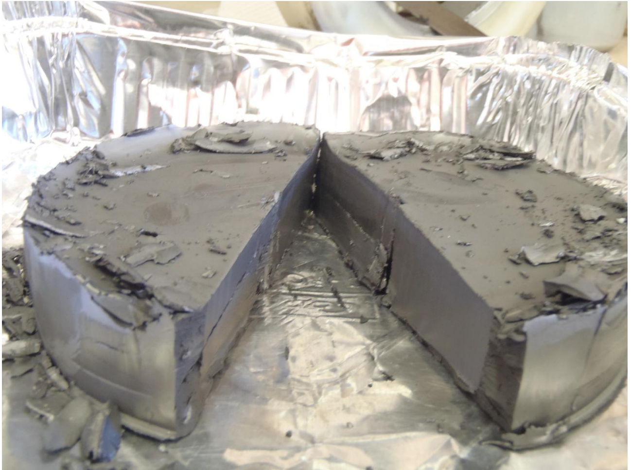
Picture 3 - 25mm PF Vittangi Graphite Concentrate Filter Cake
