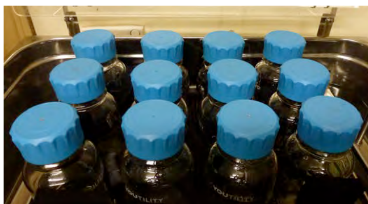
PLATE 5: Determination of Neutralisation-Potential (NP) [= Acid-Neutralisation Capacity, ANC] values for selected samples with CO 3 -C < 0.01 % using the BS EN 15875:2011 method (cf. AMIRA (2002) method) and a shaker-waterbath. Bottom photograph shows bottle-lids with a small hole for gas exchange as specified in BS EN 15875:2001.
