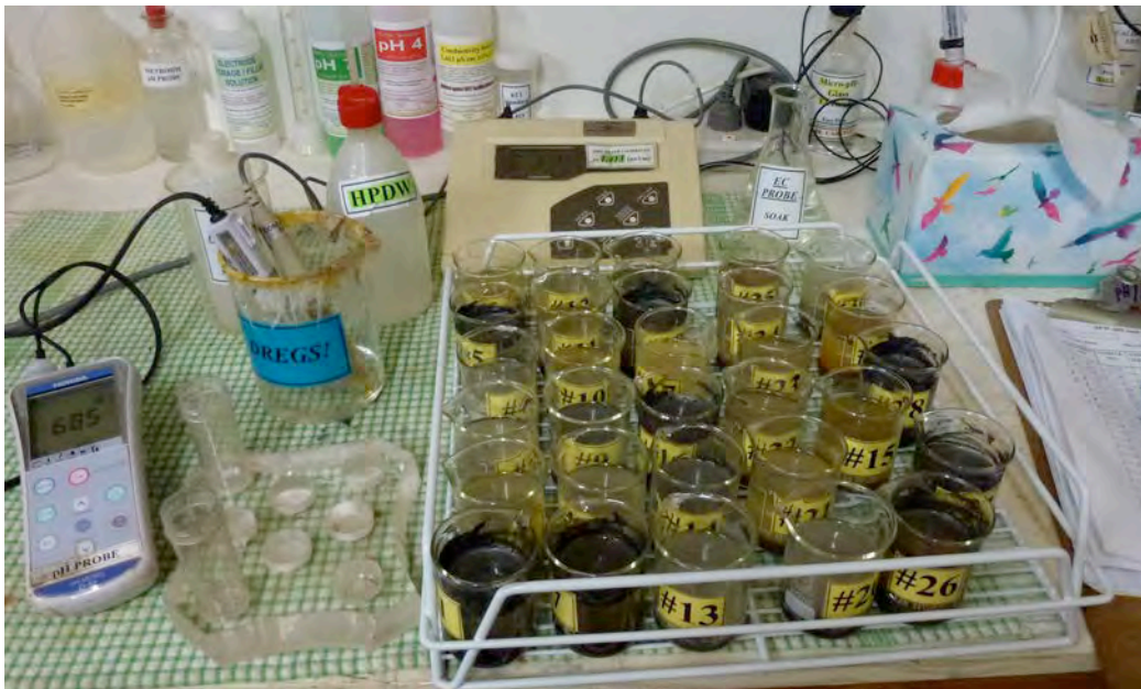
PLATE 2: Determination of pH-(1:2) and EC-(1:2) values (EC = Electrical-Conductivity). Crushed (-2mm nominal) samples aged in contact with air at room-temperature (20-22 °C) for ca. 24 hrs prior to measuring pH and EC. Supernatant-water initially decanted for EC determinations, and following return to container slurry-pH measured.
