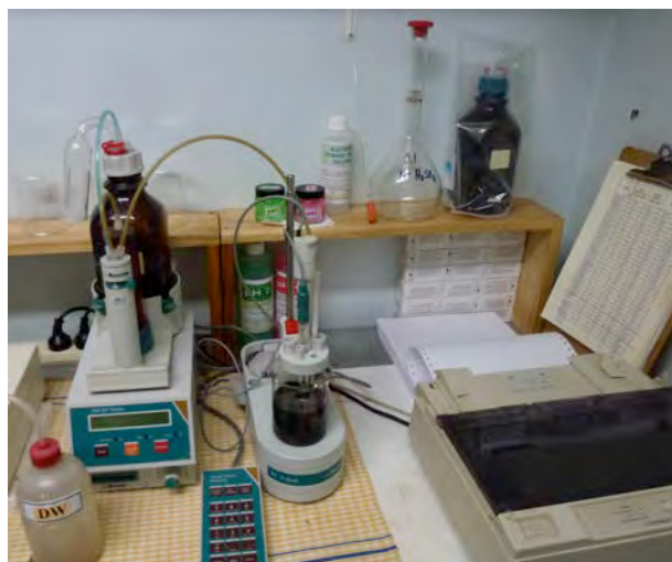
PLATE 4: Auto-titration testing using 0.1 N-H 2 SO 4 to determine pH-buffering properties of selected samples with CO 3 -C values above 0.2 %. Testing on pulps (-75 μm nominal).
