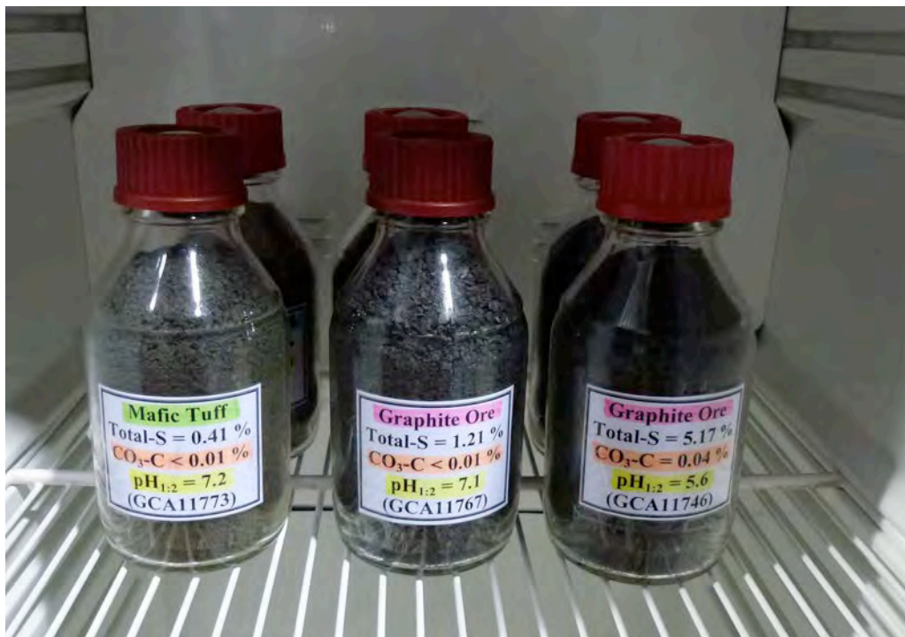
PLATE 8: Packed Oxygen-Consumption Cells (OCCs) for selected waste and ore samples, and housed in an incubator at 20.0 (+/- 0.1) °C .
