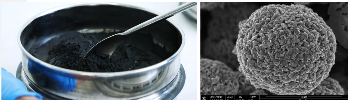
Figure 1 Talnnode®-Si under development at Talga’s R&D facilities in the UK. (L) Active anode powder preparation and (R) Scanning electron microscopy image of Talnnode®-Si particle during production.
