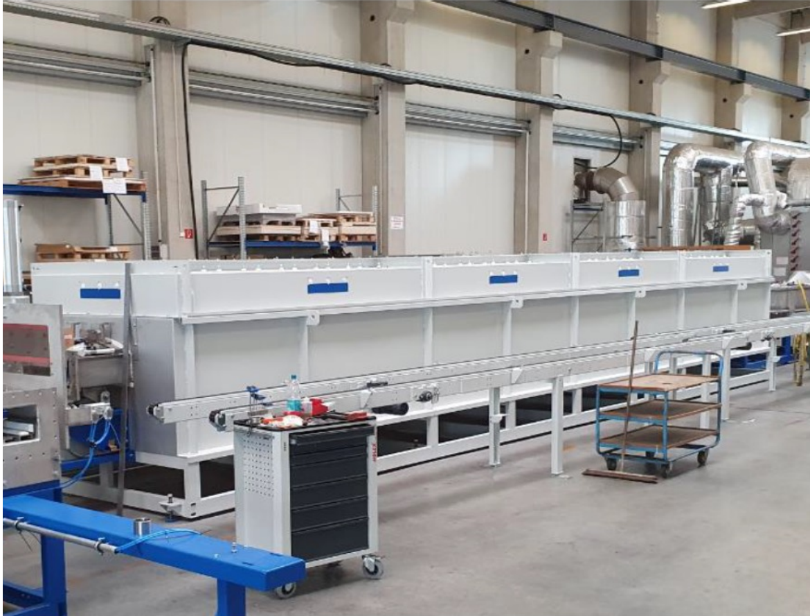
Talga EVA anode coating oven under construction
