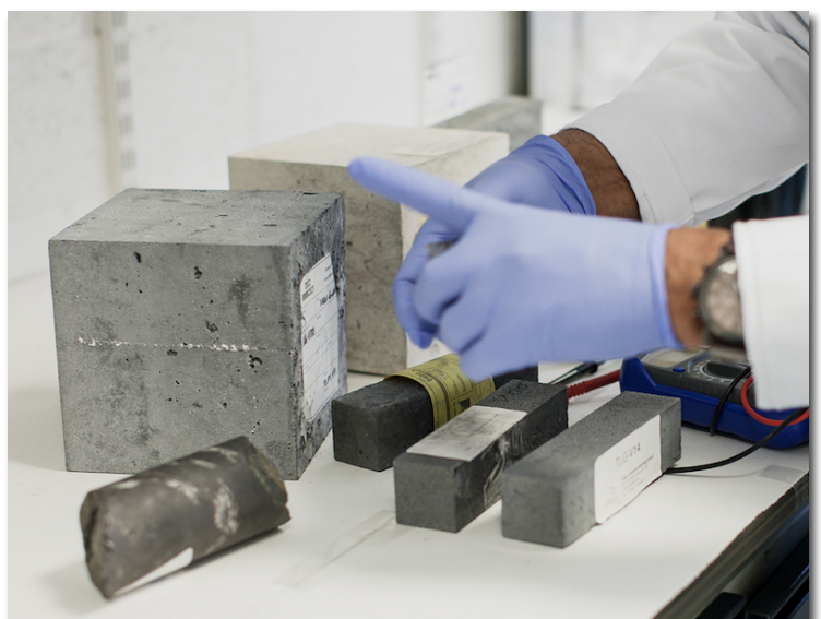
Figure 4. Concrete test samples including graphene enhanced thermally conductive and graphite containing electrically conductive specimens.
