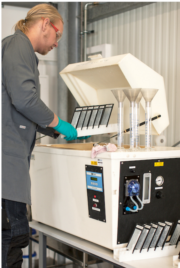
Figure 6. Salt water spray test performed by Talga Advanced Materials GmbH staff at the Company's in-house laboratory facilities in its Rudolstadt test processing facility.
