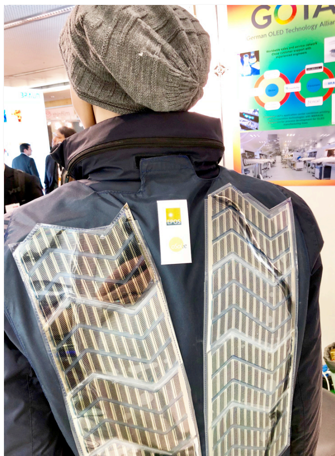
Figure 6. Conductive inks such as graphene can make flexible printed solar 'panels' and batteries, enabling the powering of mobile devices and other functions in 'wearables'.
