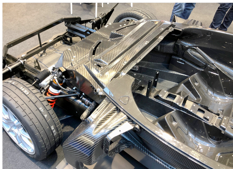
Figure 2. Light-weighting is a growing trend in vehicles that are to rely more on battery power storage than fossil fuels. Stronger and lighter carbon fibre reinforced plastic (epoxy resin) can be enabled by graphene dispersions in the resin.
