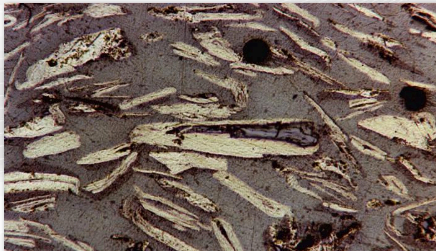
Photomicrograph: Raitajärvi Graphite Flakes 100x magnification
