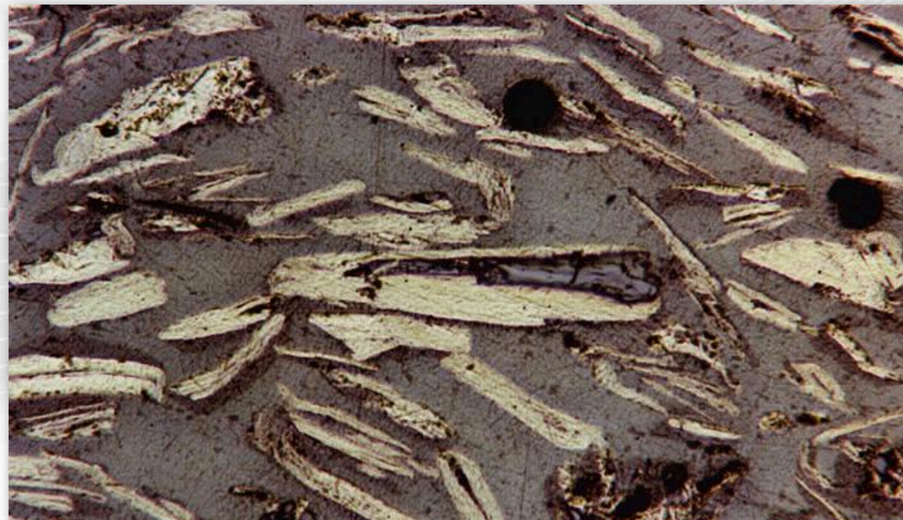
Photomicrograph: Raitajärvi Graphite Flakes 100x magnification
