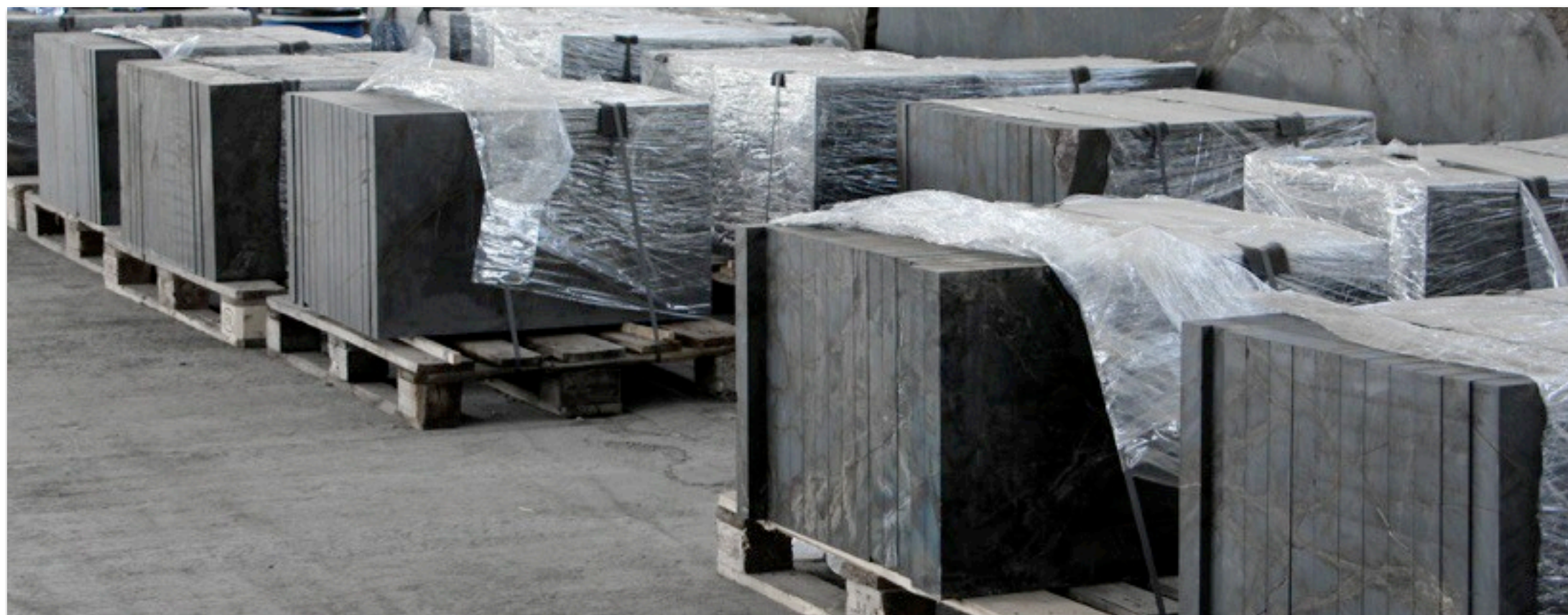
Raw ore cut into 50kg electrodes for pilot test plant processing
