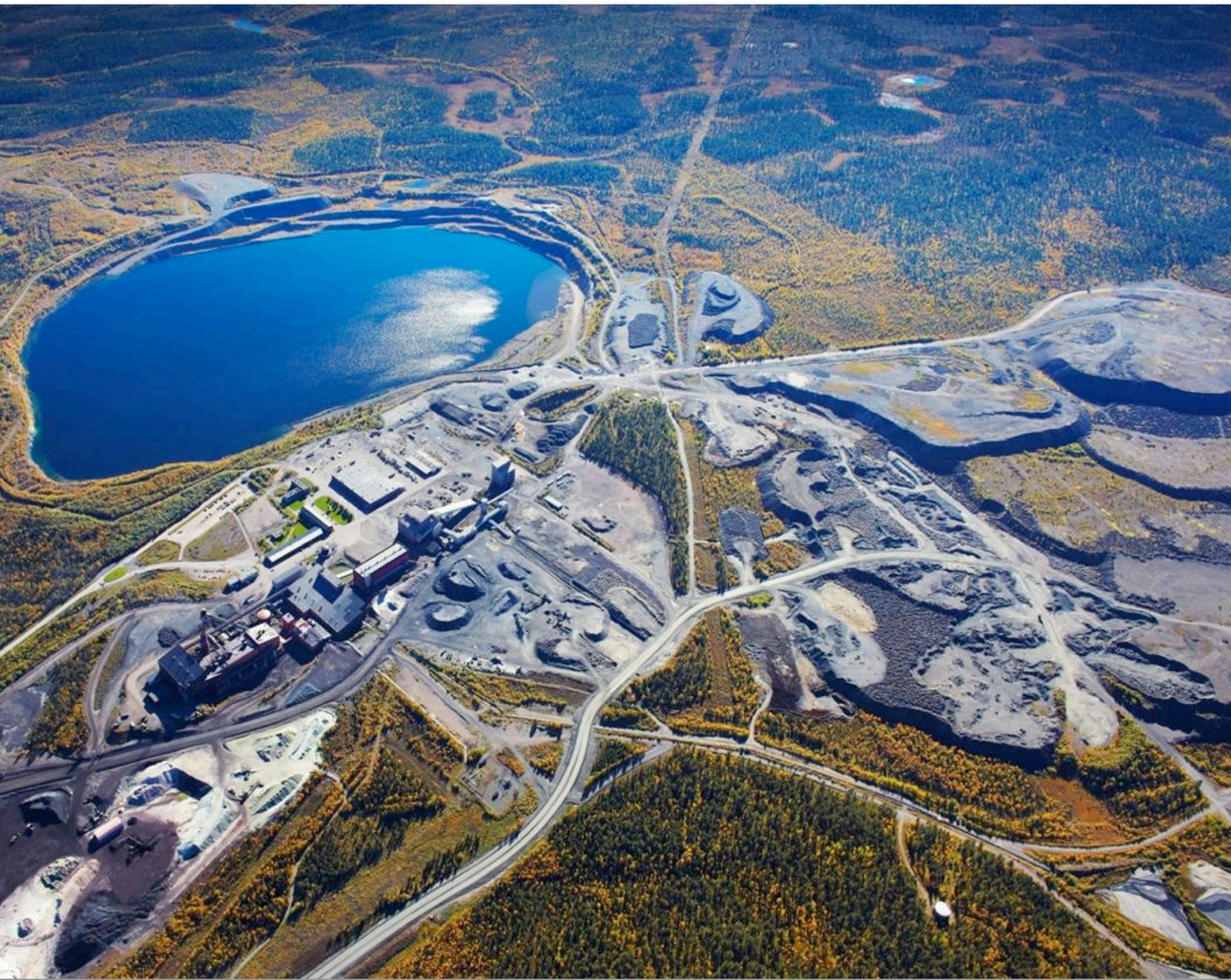
Svappavaara magnetite mine and mill owned by LKAB, approximately 30km by road from the Vittangi project and 60km from Masugnsbyn project. After an earlier phase of open pit mining the mill remained operational for Kiruna ore. The open pit is currently being dewatered to be put back into production. Photo©Fredric Alm/LKAB.
