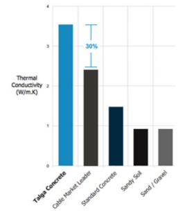
Figure 1: Thermal conductivity of Talga's concrete shows a 30% improvement over a current market leading product.
