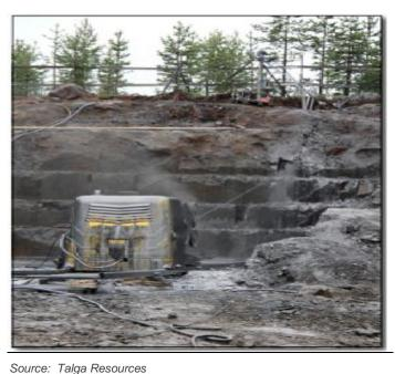
Figure 3: Preparation of first graphite ore block extraction level
