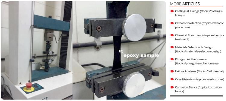
Tests were conducted on the chemical and mechanical properties of the graphene-added epoxy coatings, including the tensile strength. Photo courtesy of Talga Resources.
