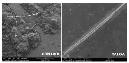
Scored coating tests found superior corrosion protection using graphene-added epoxy coatings, right, as compared to a commercial zinc-rich epoxy primer, left. Photos courtesy of Talga Resources.
