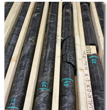
Photo 1 Graphite intersected in drillhole JALK03, Jalkunen.
