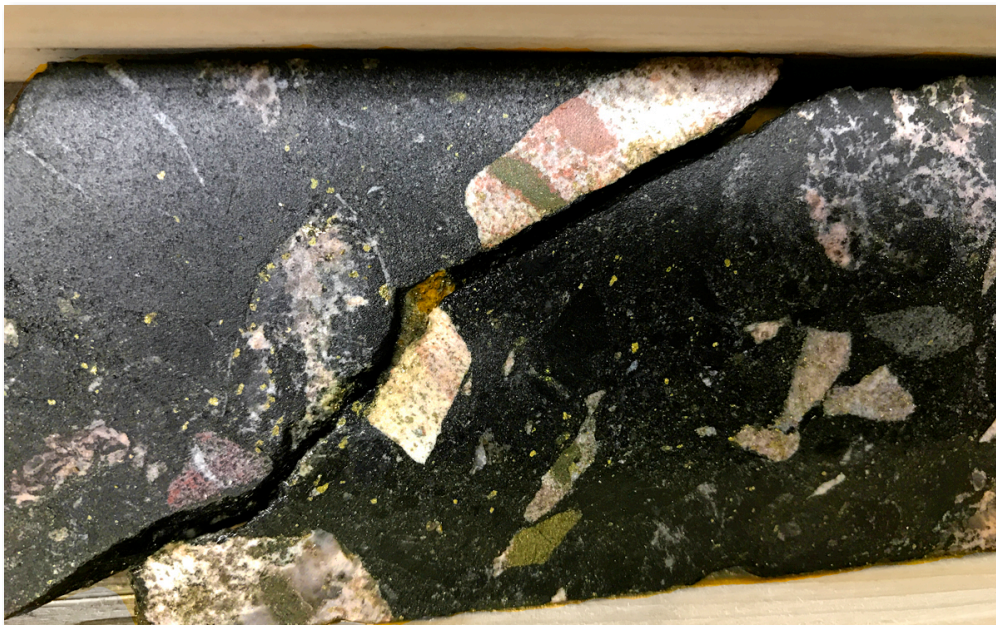
Figure 6 Lautakoski drillcore at 26m depth (LAU17001) showing disseminated copper-bearing sulphides in magnetite rock supporting breccia clasts with both vein and disseminated mineralisation.
