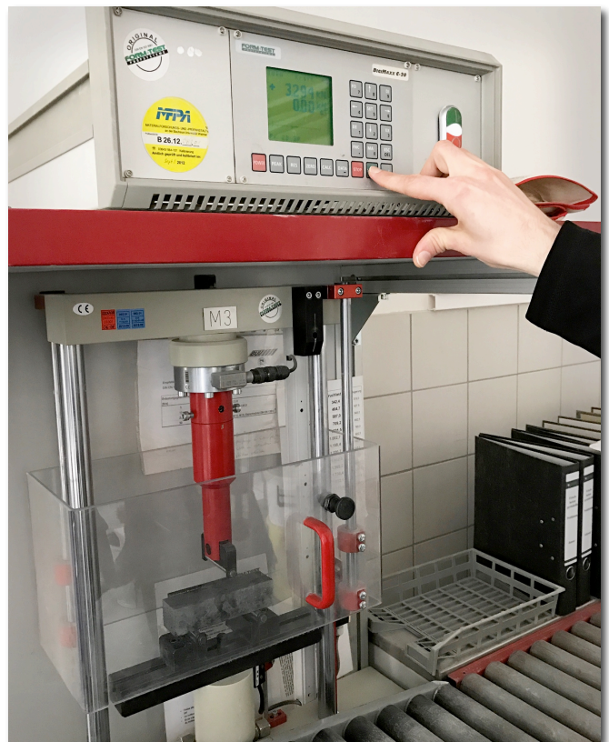
Figure 1 Talga concrete prototypes during compression (L) and flexural strength (R) trials at Betotech, Germany.
