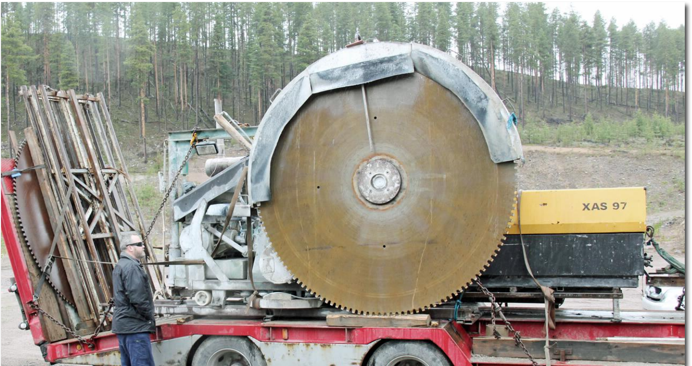
Figure 7 - Part of the graphite ore block cutting equipment arrives on site.
