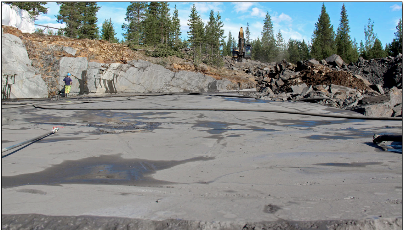
Figure 5 Preparation of first graphite ore block extraction level for 2016 at Talga's Vittangi project.
