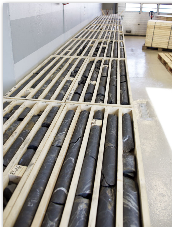
Figure 1 Graphite in drill core from Niska North (NUN19010); refer cross-section Fig 2 and Table 1 below for details.
