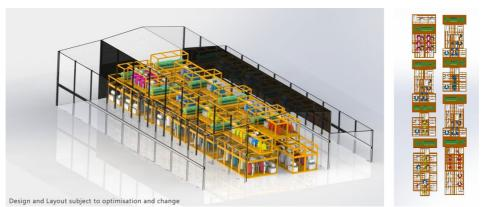
Figure 2. EVA plant process modules layout option (schematic).
