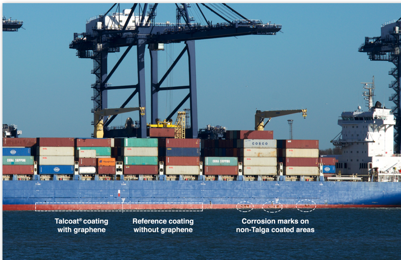
Figure 2. Port-side Talcoat® application area and reference area after 15 months service on Robin 1
