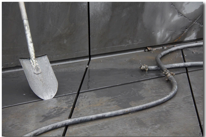
Figure 3 - Closer view of graphite ore showing amenability of mining method in precisely preparing the ore blocks and the homogenous nature of Vittangi graphite mineralisation.
