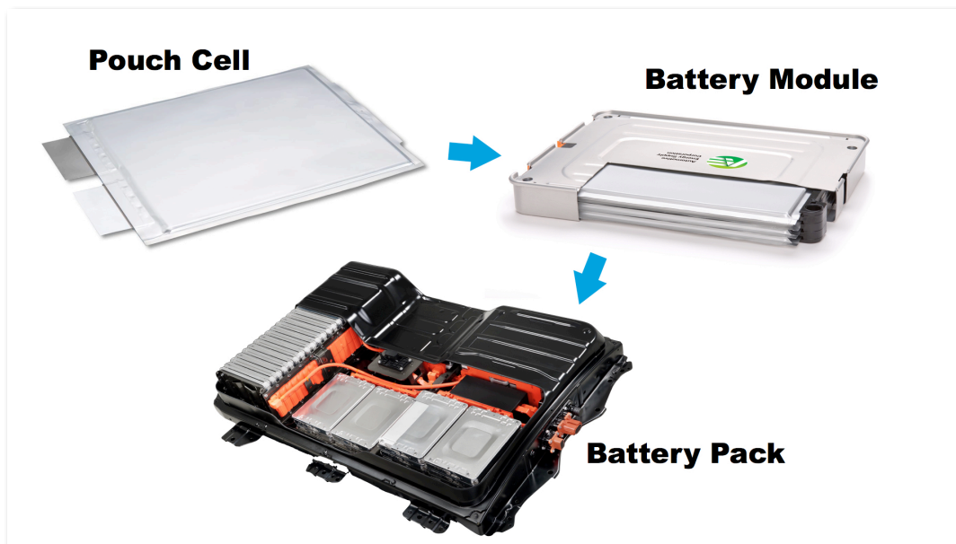
Figure 2 Packaging of pouch cells in current commercial electric vehicle battery packs eg. Nissan Leaf, BMWi3
