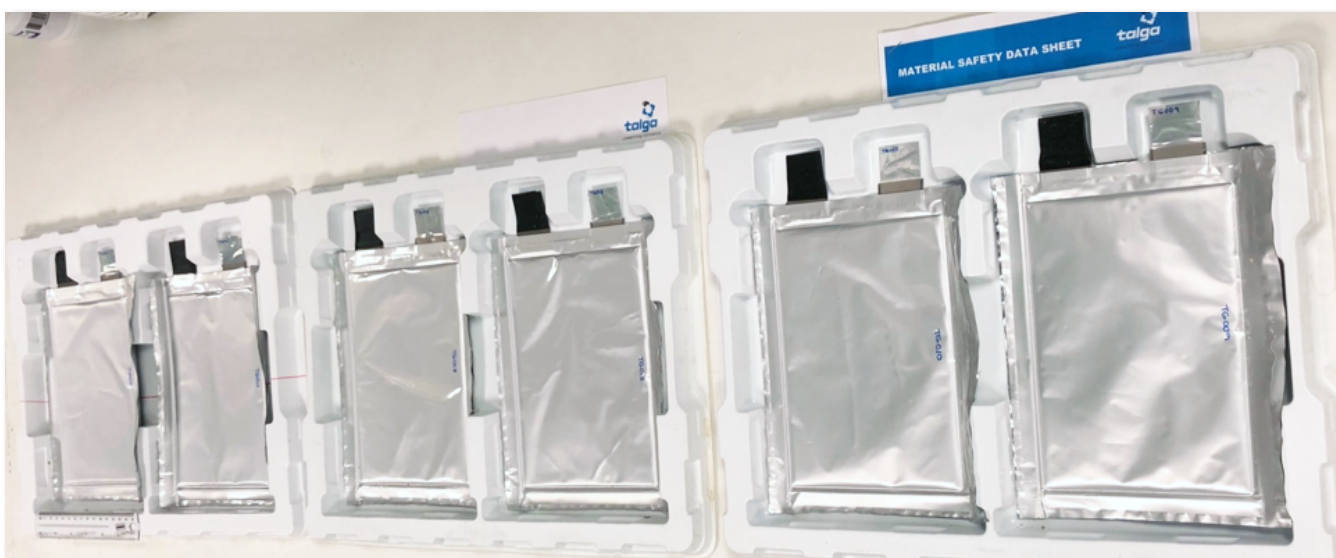
Figure 1 Full scale pouch cells (A5) targeting 4Ah capacity containing Talga graphite anode and NMC cathode.
