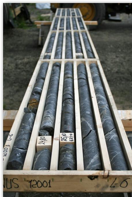
Figure 2. Talga's maiden drillhole NUS12001 showing part of high grade graphite unit.
