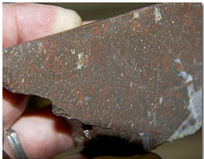
Fig 3. Kiskama drillcore showing IOCG style mineralisation
