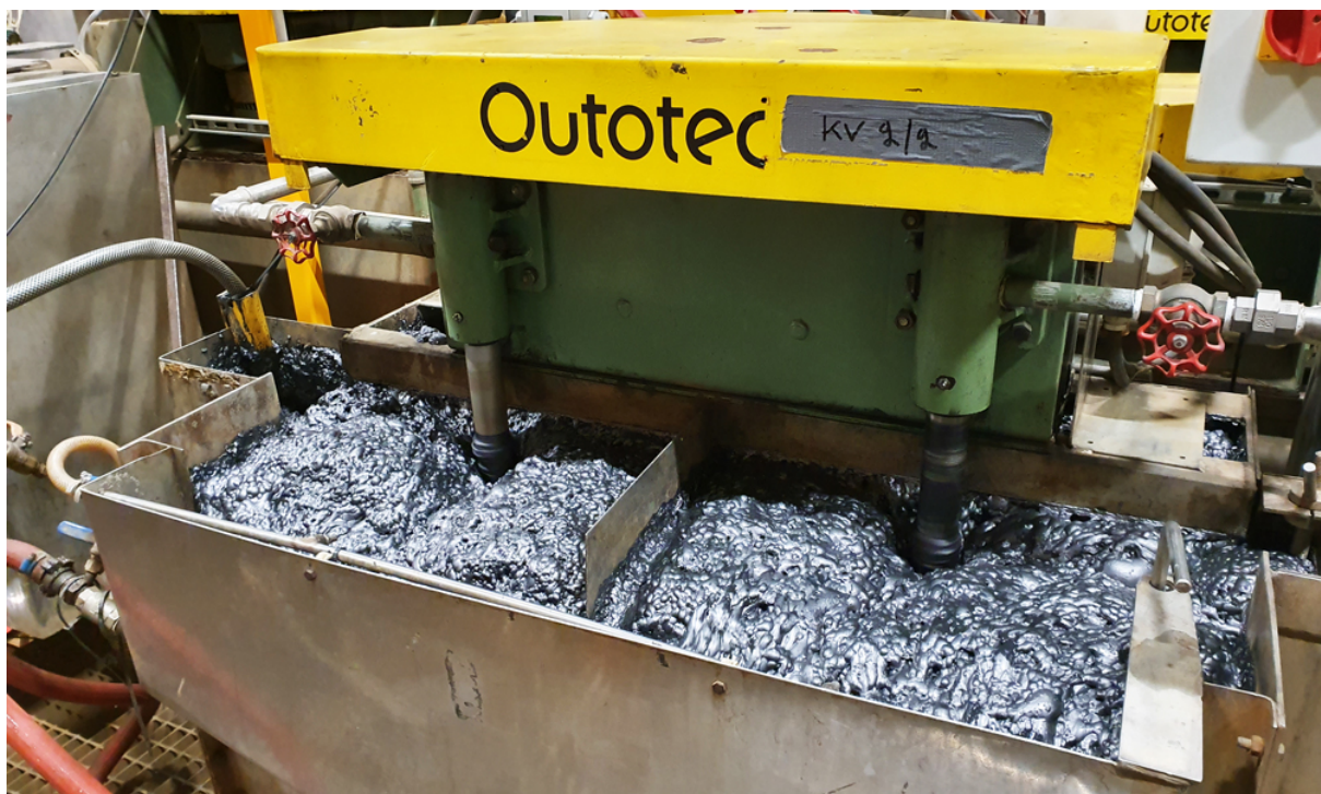
Figure 5 Talga concentrate being produced from 60t bulk sample pilot early 2020.
