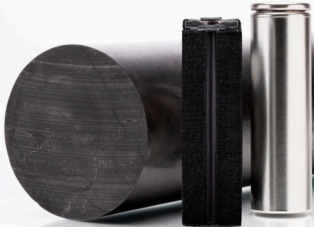
Drillcore from Talga's Vittangi graphite deposit and Li-ion battery sectioned to show graphite anode material interior ©Talga Group
