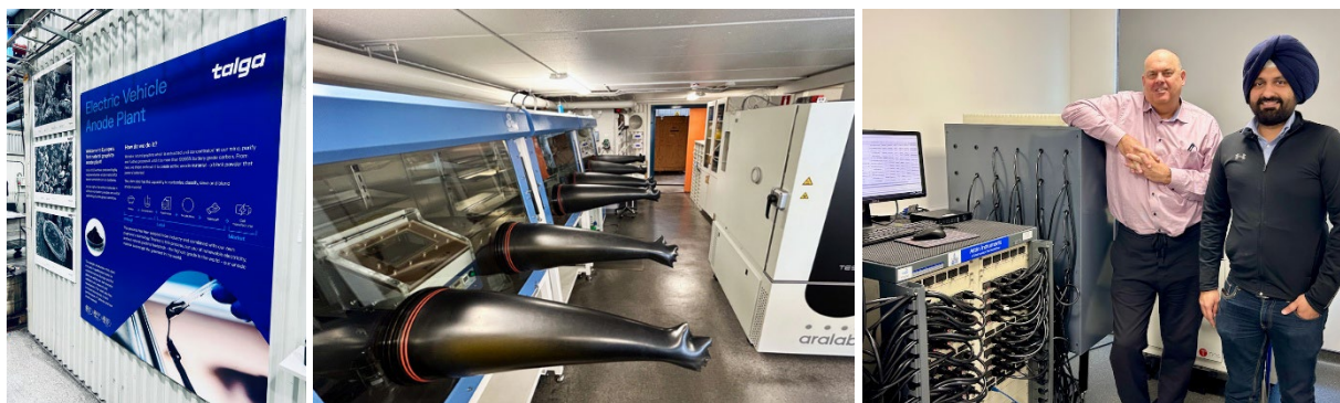
Figure 2 Information and anode QC/QA lab at Talga’s EVA plant in Luleå, Sweden (L-C), and part of cycling test room for Talnode® products at Talga’s battery Centre of Excellence in Cambridge, UK (R).
