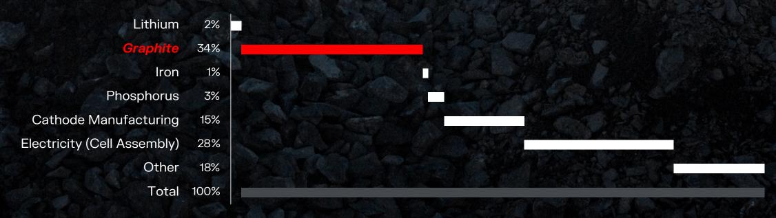
LFP Battery Cell — GWP Contribution Analysis (CO<sub>2</sub>, impact per kg)
