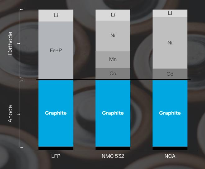
Graphite is used as the anode of almost all Li-ion battery types due to performance, safety and cost
