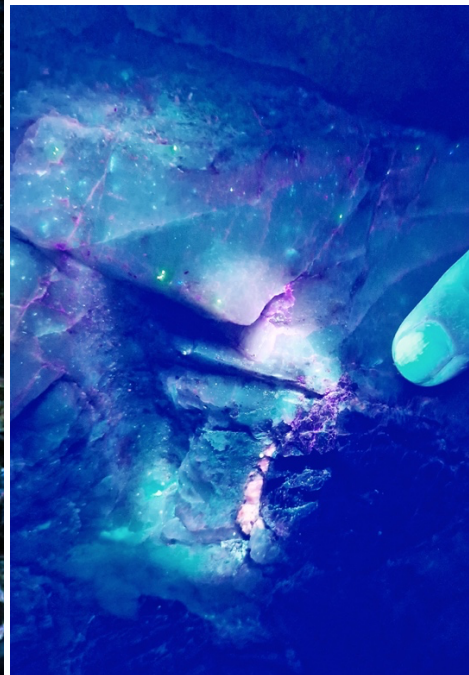
Figure 1 Talga geology team conducting night-time UV prospecting for lithium minerals at the Aero Project in northern Sweden. Positive observations are recorded and marked with pink tape for collection the next day.
