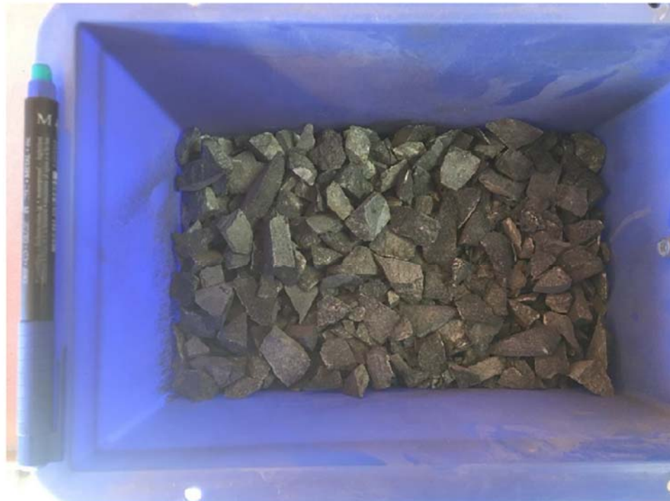
Figure 2: Used size fraction for the large kinetic tests.
